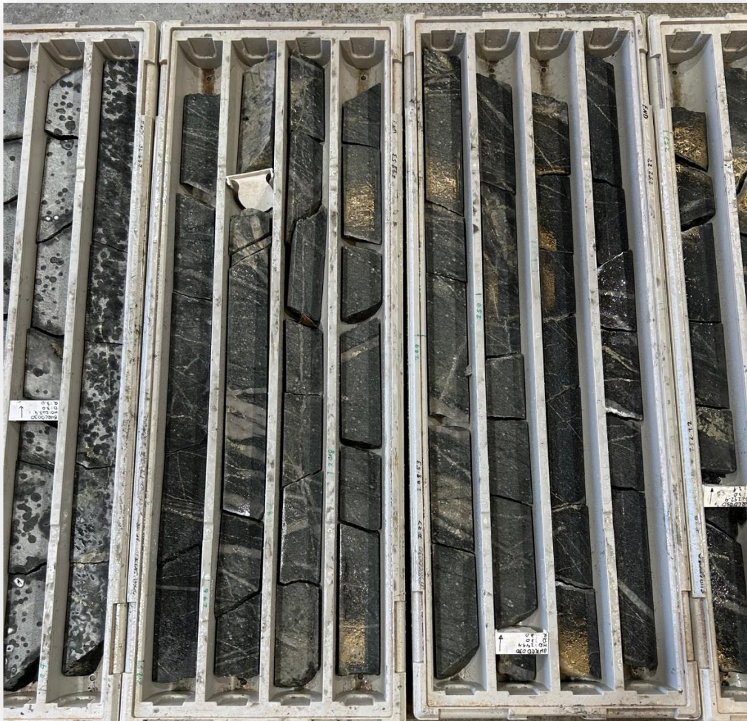
Figure 2: Photograph of core from BHRC030, 244-253m showing numerous plagioclase-phyric dacitic porphyries with sulphide minerals (pyrite-chalcopyrite) hosted in cross-cutting veins
