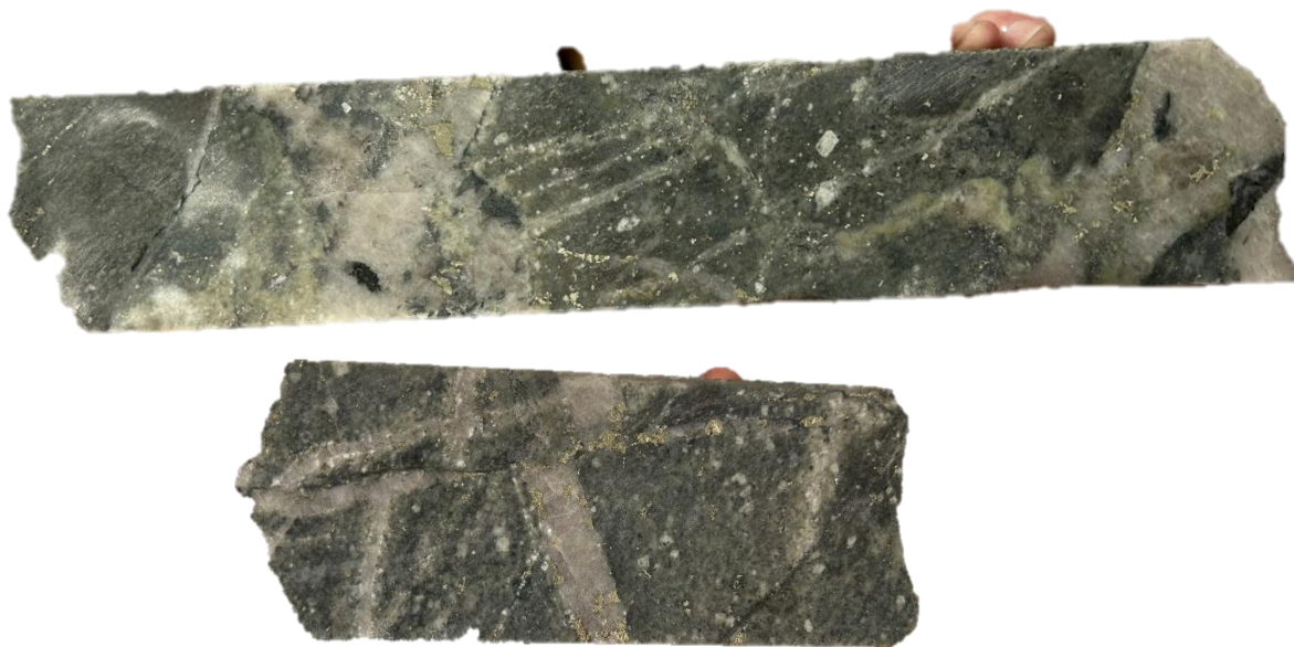
Figure 3: Photographs of core from BHRCD018 showing sulphide minerals hosted in cross-cutting veins
