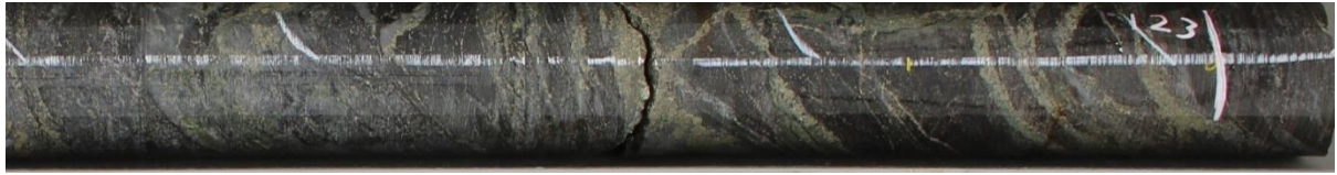
Figure 1: Photograph of core from BHRC030, 123m showing quartz-pyrite veins \pm chalcopyrite-molybdenum
