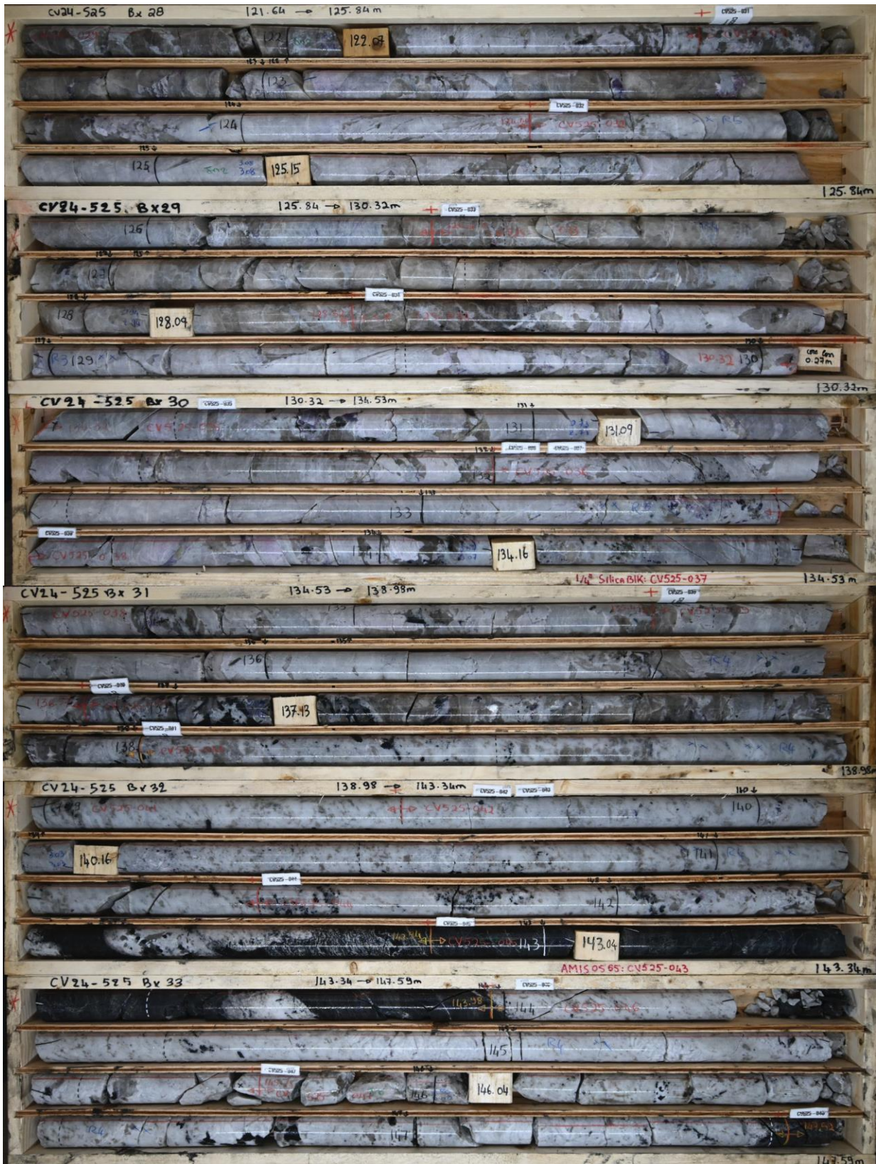
Figure 5: High-grade spodumene pegmatite drill intercept from the Vega Zone at the CV13 Spodumene Pegmatite, assaying 9.7 m at 5.16% \text{Li}_2\text{O} (128.3 m to 138.0 m) in drill hole CV24-525.
