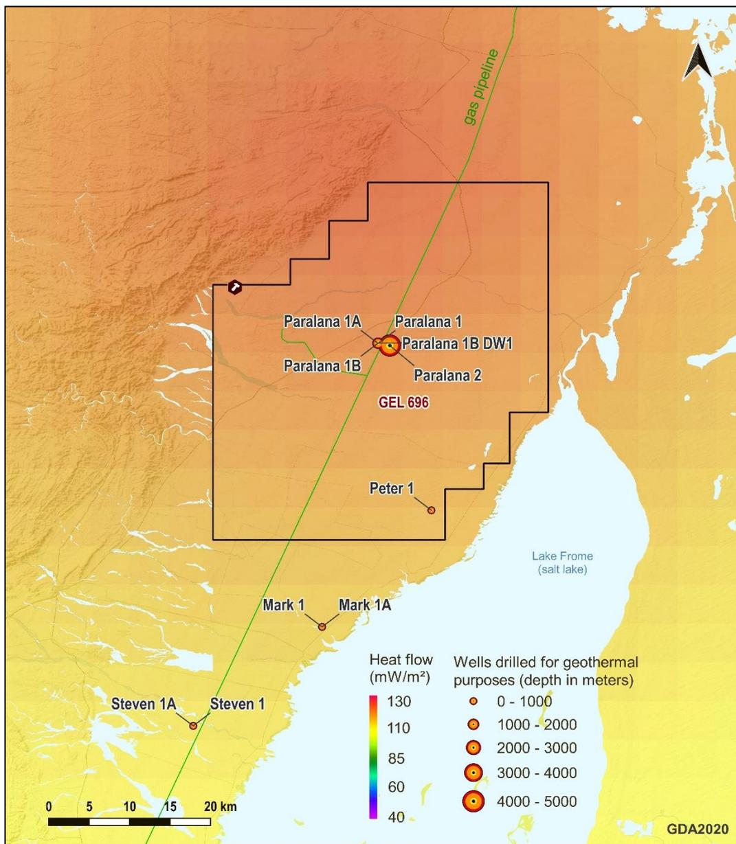
**Figure 3:** Paralana Project contains multiple geothermal wells drilled between 2,000m to 4,000m depth
