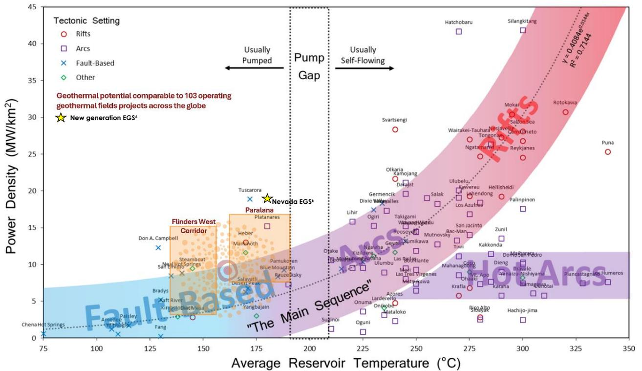
**Figure 2:** Potential Power Density Range of EE1 Projects<sup>10</sup> compared to other global Geothermal projects<sup>11</sup> – orange box are current indicative bands of the power density range for EE1's South Australian projects
