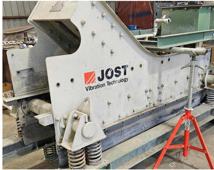
Figure 2: Vibrating Screen and other ancillary processing equipment associated with the Gravity Circuit
