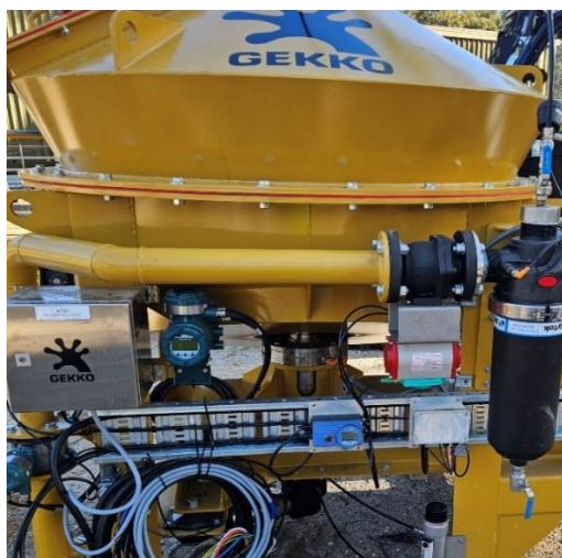
Figure 1: Wolff Batch Centrifugal Concentrator – coarse gold gravity collector
