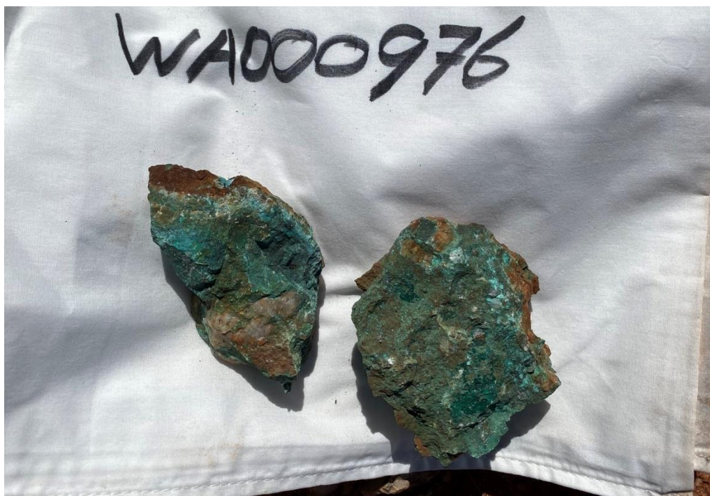
Figure 12 Sample WA000976 from Tiberius showing malachite mineralisation which assayed 34.6% Cu and 0.26% Pb.
