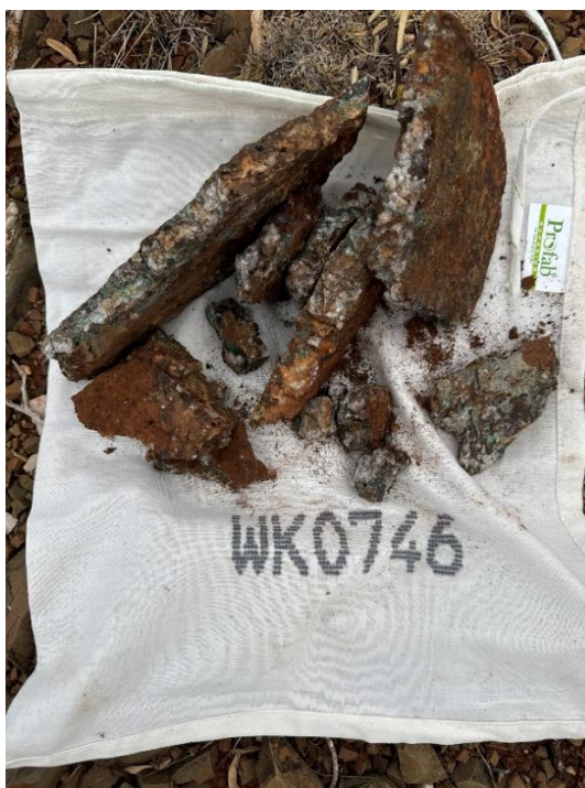
Figure 1. Sample WK0746 (11.5% Cu). Mineralised quartz vein including chalcocite and malachite copper minerals.
