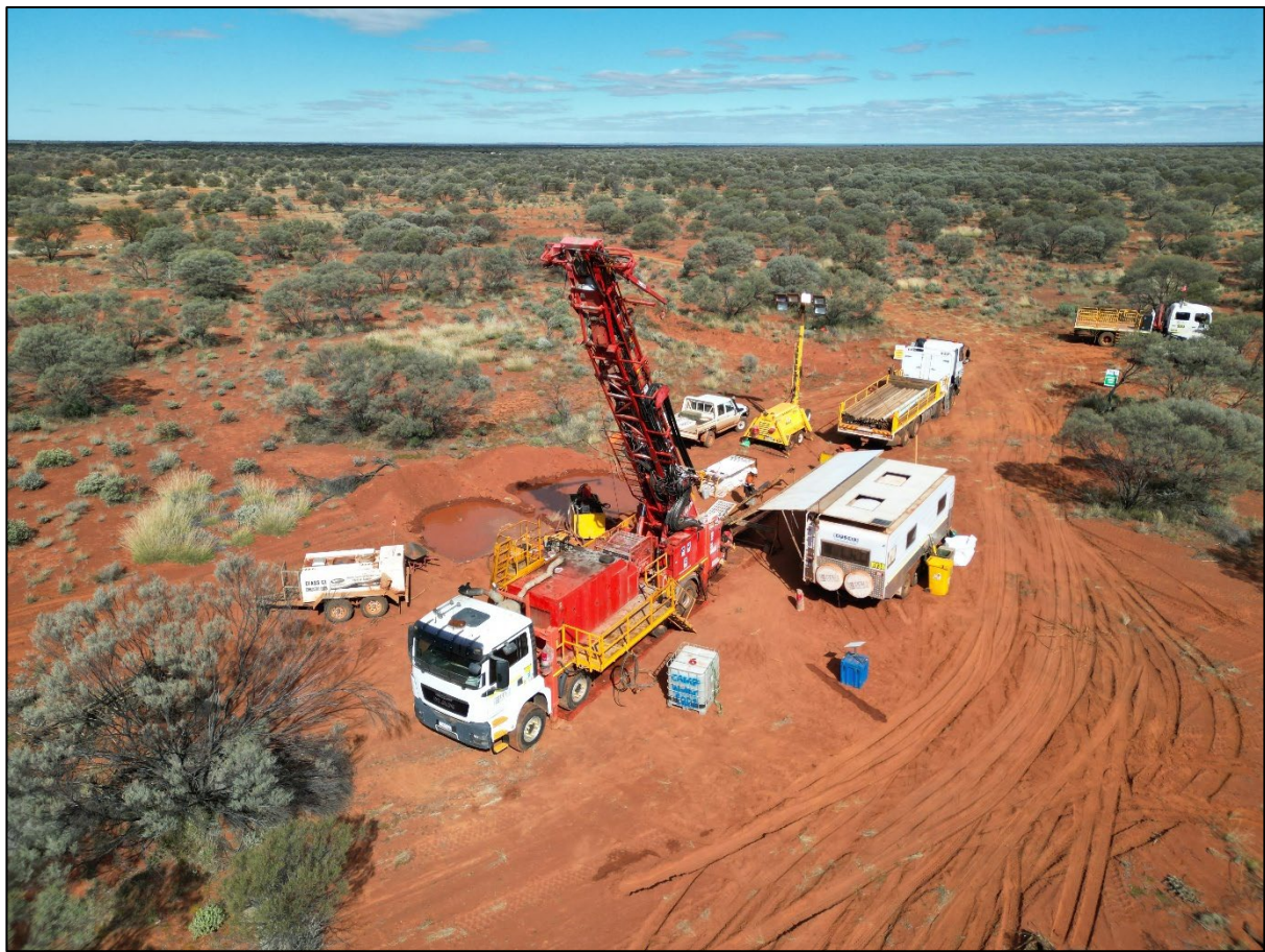
Figure 4: Diamond drilling rig on the first of two planned diamond holes (24YRLEIS0001) testing the NEG Prospect
