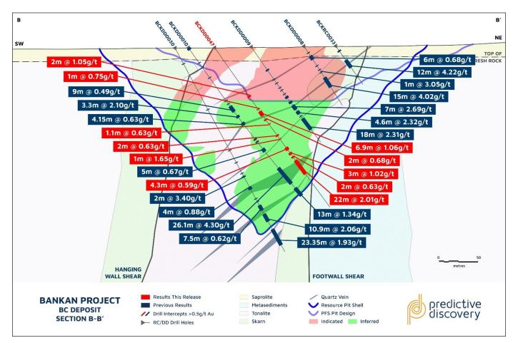
Figure 4: BC cross section B-B'
