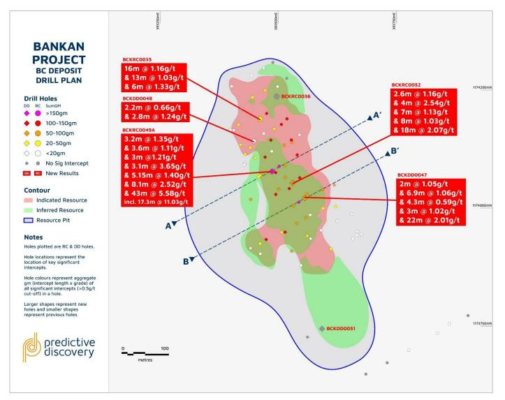
Figure 2: BC drill plan
