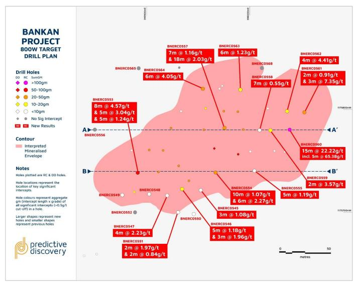
Figure 5: 800W drill plan
