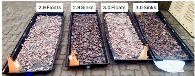
Figure 7. DMS test work sample trays showing sinks (dark) and floats (light).
