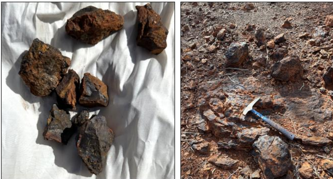
Figure 4: High grade rock chip BB7 60.63% Fe (left image), and area of enriched outcrop located 676,420mN and 7,150,310mN (right image).
