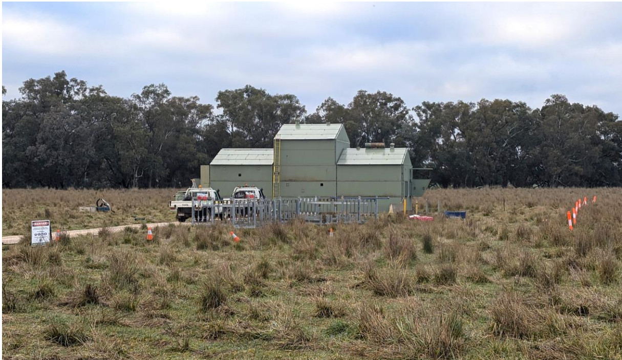
Figure 4. Photo of Deepcore's acoustic shed housing the rig drilling hole SGLD0001, and paddock mats to protect ground cover.
