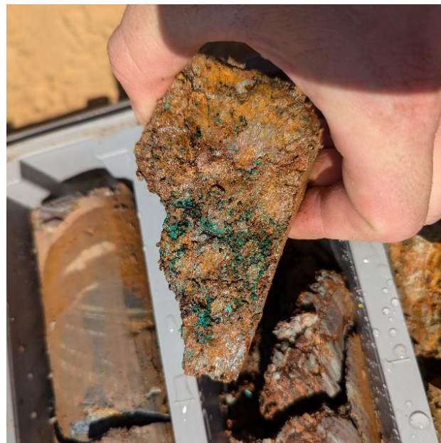
Figure 3: Photo of secondary copper carbonates in the gossanous horizons from ~14m depth in KMDD004 which is located ~100m up dip of the 50,000S off-hole conductor.
