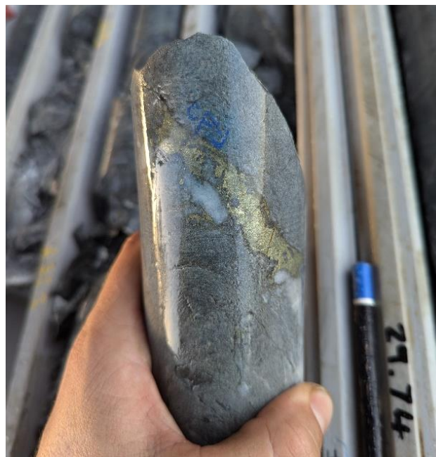
Figure 4: Photo of Grant's style Cu-Au veining from ~30m down hole in KMDD005 showing chalcopyrite as the primary sulphide.
