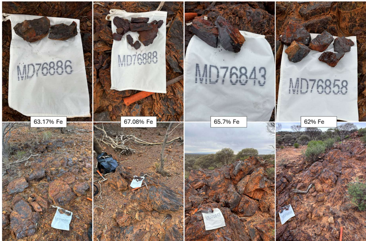
Figure 11. Example rock-chip sample and outcrop photos. (see Annexure B for location data)
