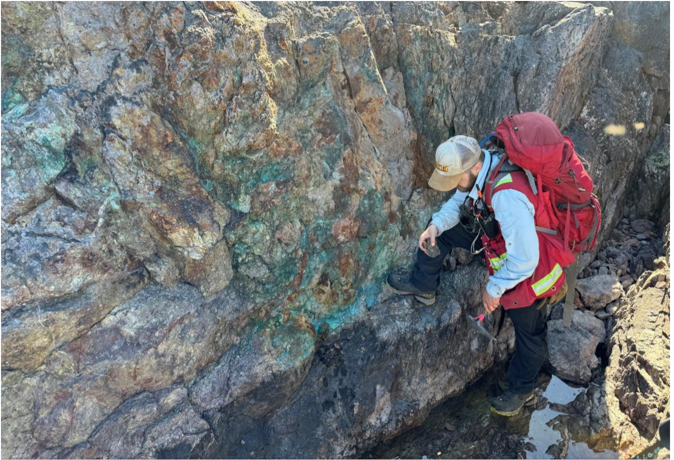
Figure 3 - Example of malachite-stained fracture surface at the Spud North trend. (Sample F005906).
