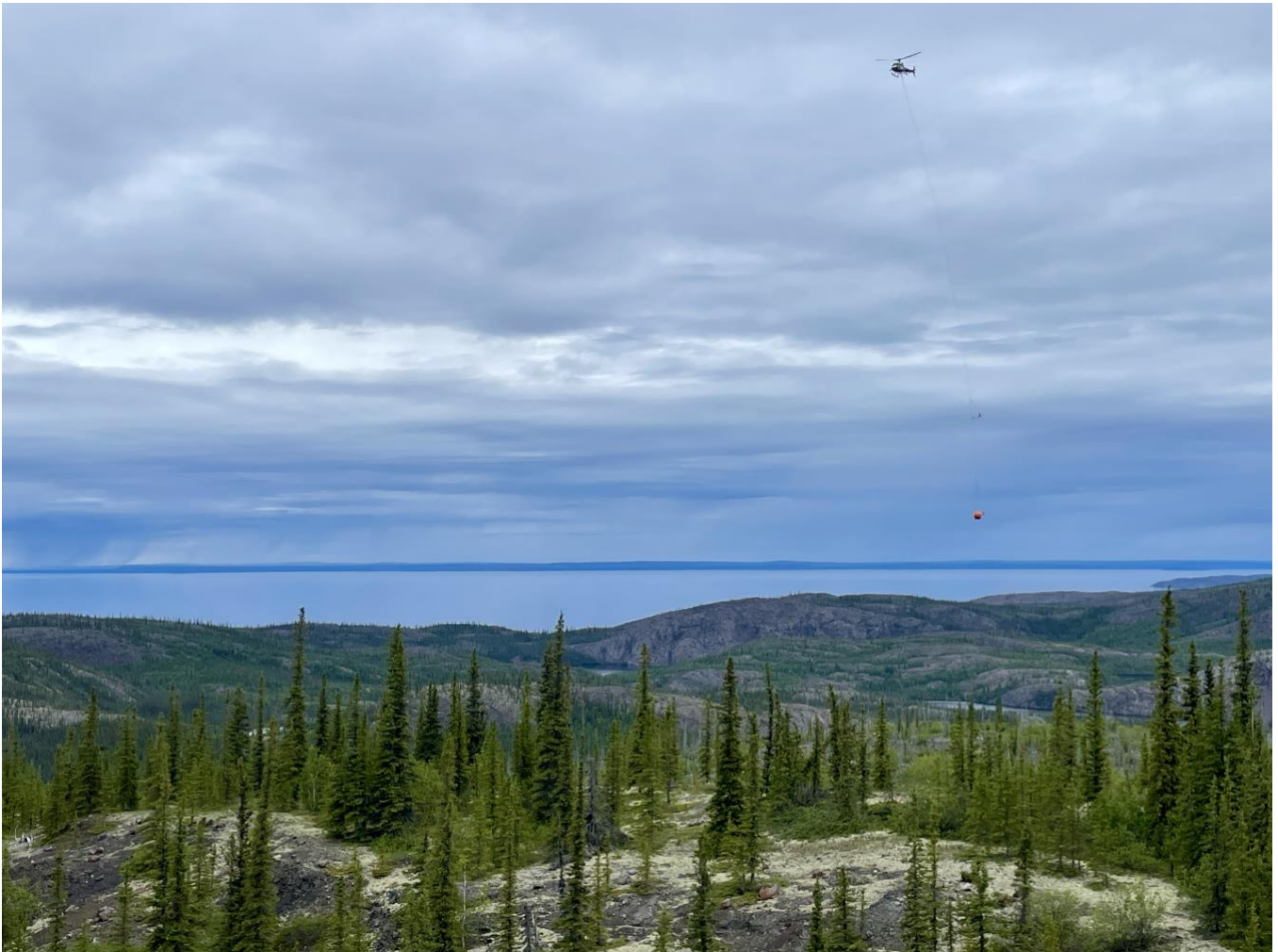
Figure 6 - Expert Geophysics Aerial Helicopters utilizing the latest MobileMT technology undertaking Aerial geophysical survey over the Cleaver IOCG target collecting valuable magnetic and conductivity data.
