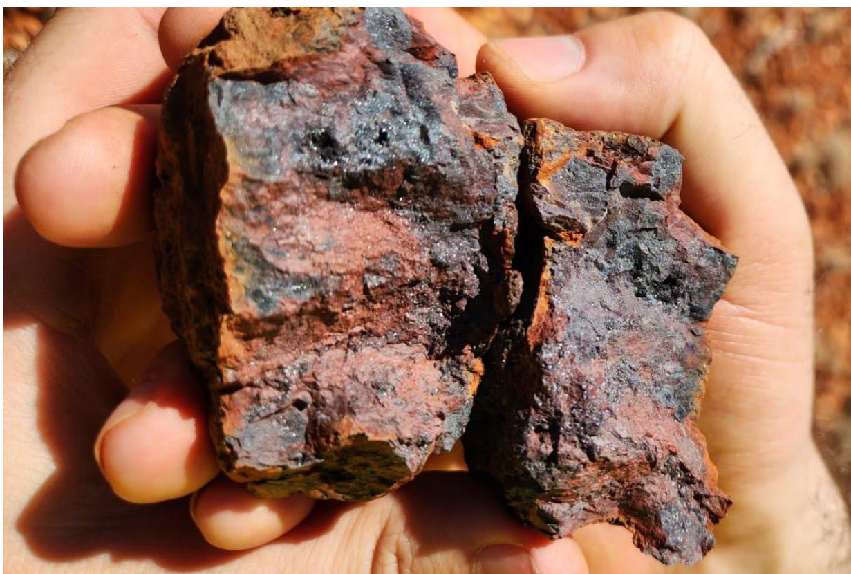
Figure 1: Hematite scree sample from Goldsworthy Project- Southern Gravity Target
