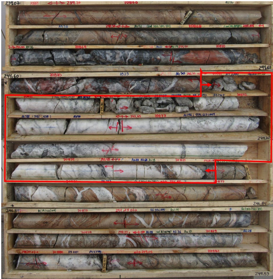
Figure 5. Hole CBD145 drill intercept of 3.1m @ 332g/t AgEq (192g/t Ag & 1.7g/t Au) hosted solely within a pre-mineral dacitic dome.
