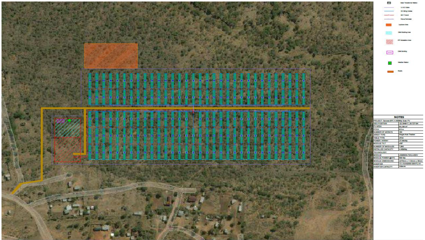
Figure 3 – Proposed layout of the 4MW solar plant within the Serowe Energy Hub and power line route to the nearest power corridor
