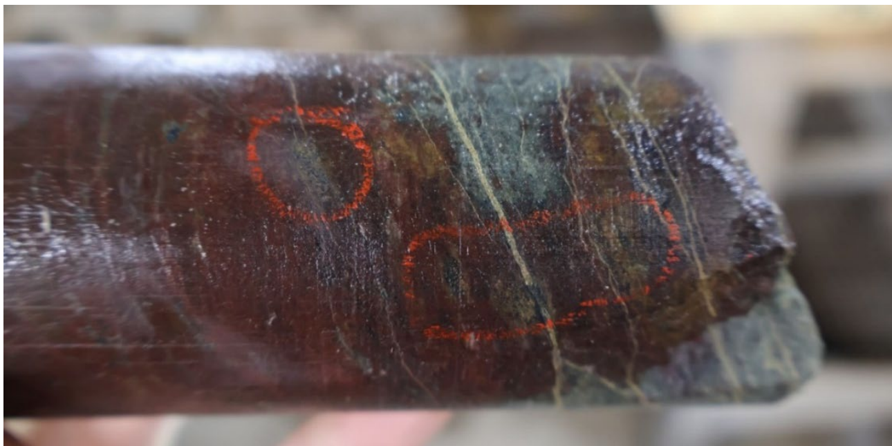
Figure 7: GC24-04: Close-up of uranium mineralisation in core sample with peak radioactivity (8,662 cps) assay value of 757ppm U3O8 at 107.87 m.
