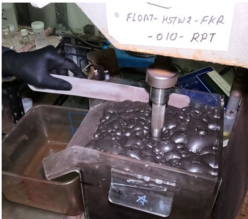
Figure 1 - Bench scale flotation testwork at Bureau Veritas laboratories, Adelaide
