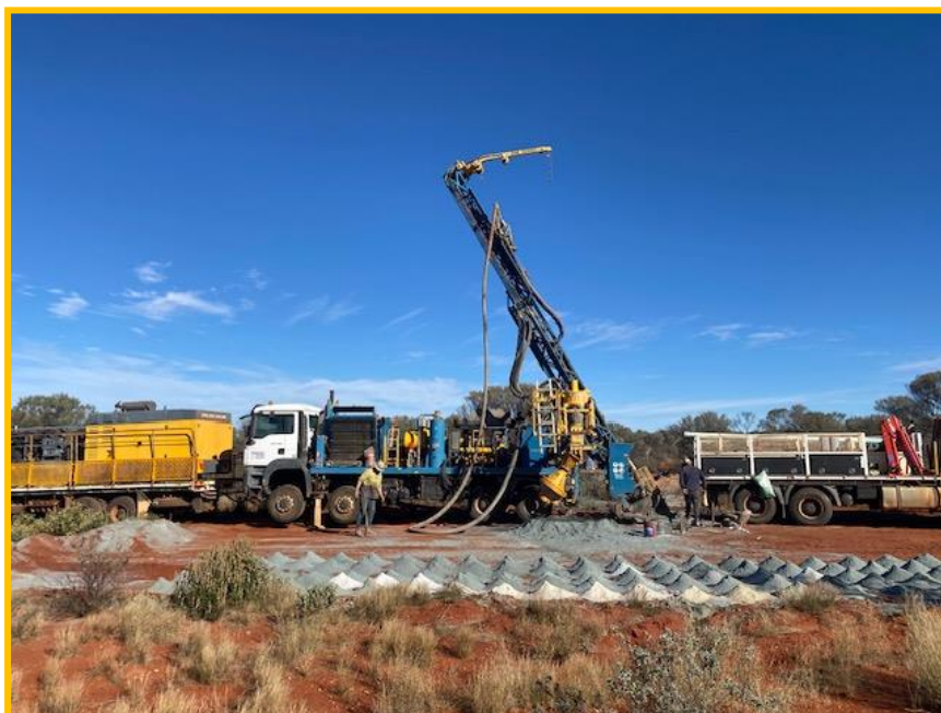
Photo 1: Stage two gold drill hole IVRC039 drilling and sampling in progress.
