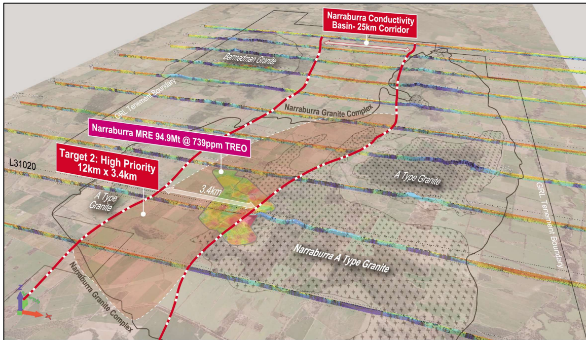
Figure 3: Perspective view looking north-west, showing the 25km long, north-south trending Narraburra Conductivity Basin. The CDIs are shown as the east-west trending pseudocolour lines, with flight line 31020 directly crossing the Narraburra Deposit. Target 2 is considered a high priority regional exploration target where conductive regolith overlaps with interpreted A-Type per-alkaline granite (source rock for REE mineralisation). Background Image: Google satellite.
