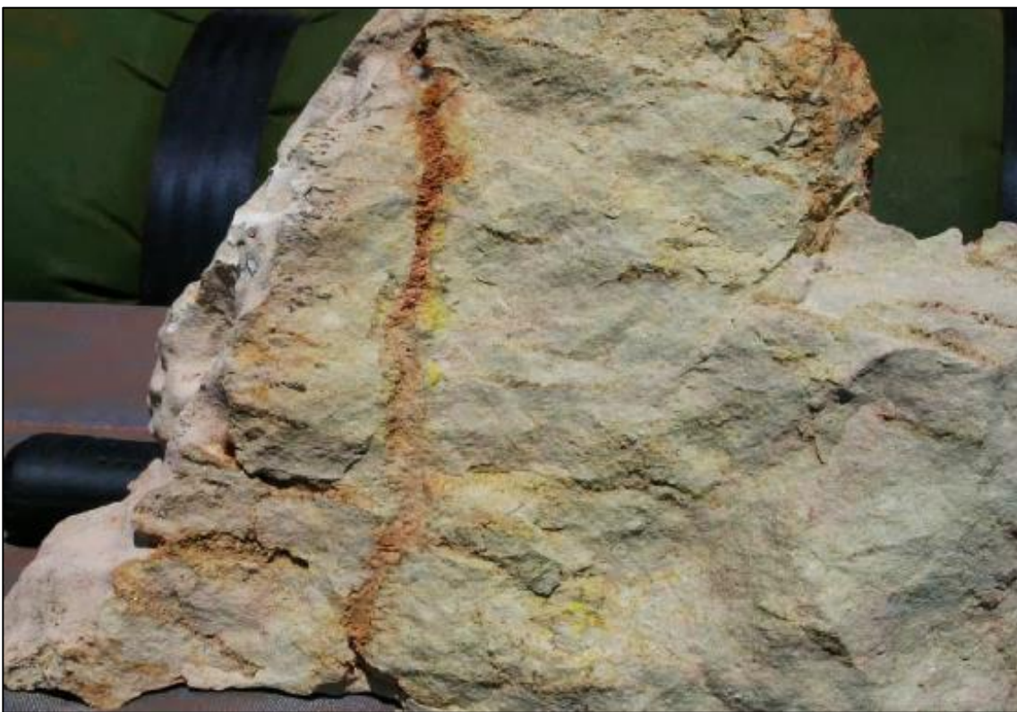
Figure 6: Carnotite (uranium) mineralisation (yellow mineral) in porous sandy limestone from the Ben Hur prospect.
