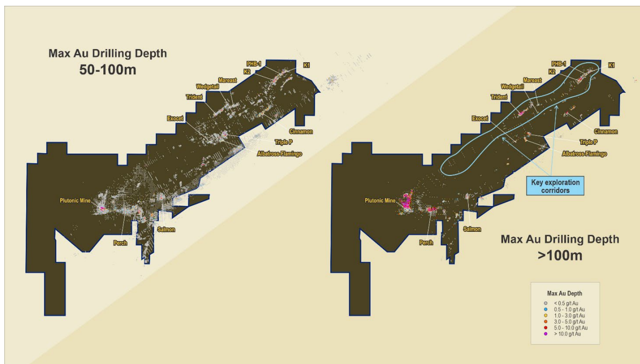
Figure 8: Plutonic gold belt showing mineralisation below 100m versus drilling density below 100m
