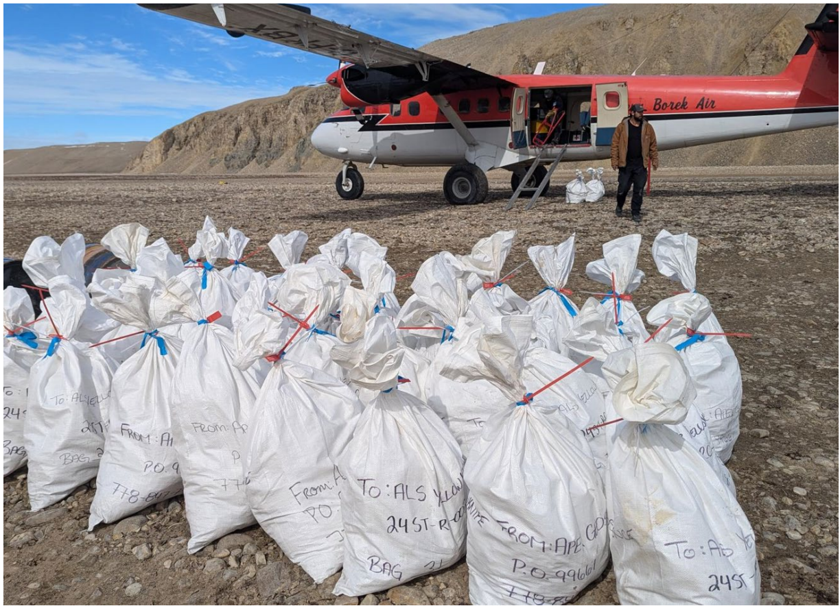
Figure 1: Reverse Circulation (RC) drill samples at the Storm Project, Nunavut, being loaded for their journey to the laboratory in Yellowknife for processing.
