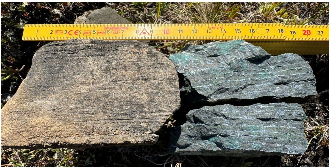
Figure 4 - Example of thinly bedded fine-medium grained sandstone (left) and a similar grained sandstone with chalcocite veining following the proto-bedding planes of the sedimentary rock (right) (Sample F005932)
