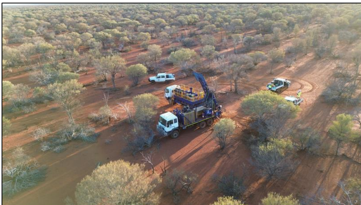
Figure 2: Aircore geochemical drilling in typical soil-covered terrain at the Yarri Project. Extensive soil cover means that any previous surface geochemical sampling can be considered to be largely ineffective.
