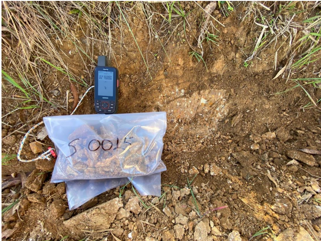
Figure 2 – Portao Verde surface sample, weathered porphyritic volcanic – 2,489ppm TREO (sample ID S0015).
