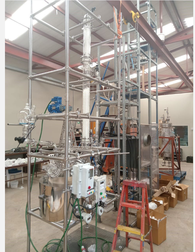
Image: Distillation column for Globe's Pilot Plant under construction at Resonant Group's facility in Johannesburg, South Africa
