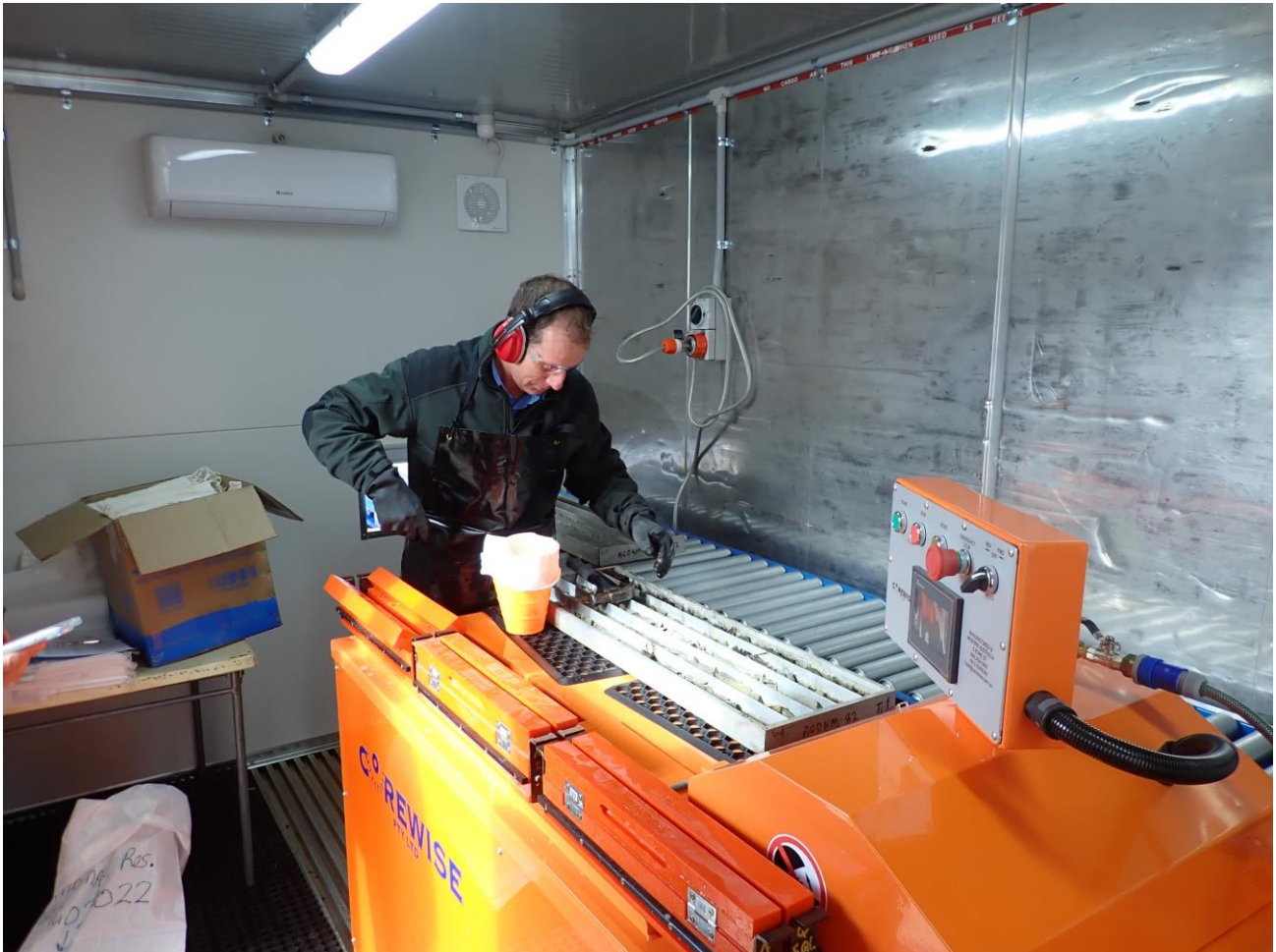
Figure 3. Magmatic personnel resampling historic core from the Myall Project.
