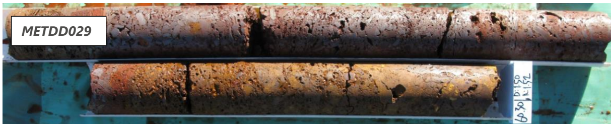
Figure 9: Drill hole METDD029 from 58.8m to 60.3m showing typical canga above Fe enriched hardcap within the Dales Gorge Member
