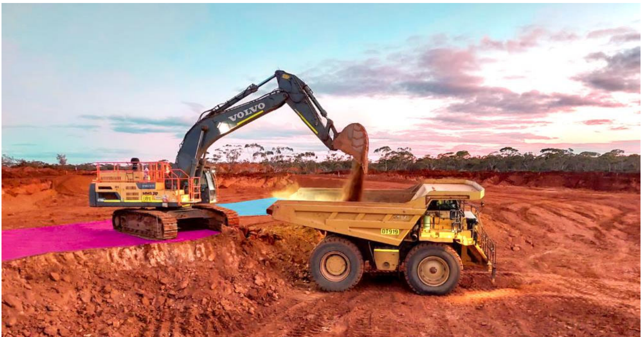
Figure 1: First Ore being loaded at the Myhree open pit (pink >3.0g/t Au, blue <3.0g/t Au).
