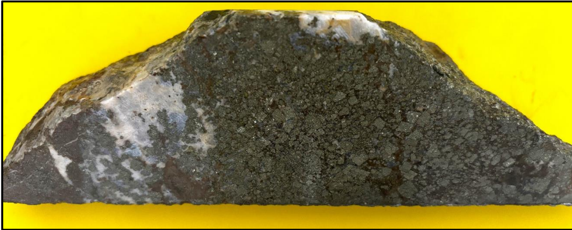
Figure 9. Drill core from 242.1m in ZRSD24147, assaying 4.5g/t Au Eq (2.3g/t Au, 1.2% Cu and 5g/t Ag)
