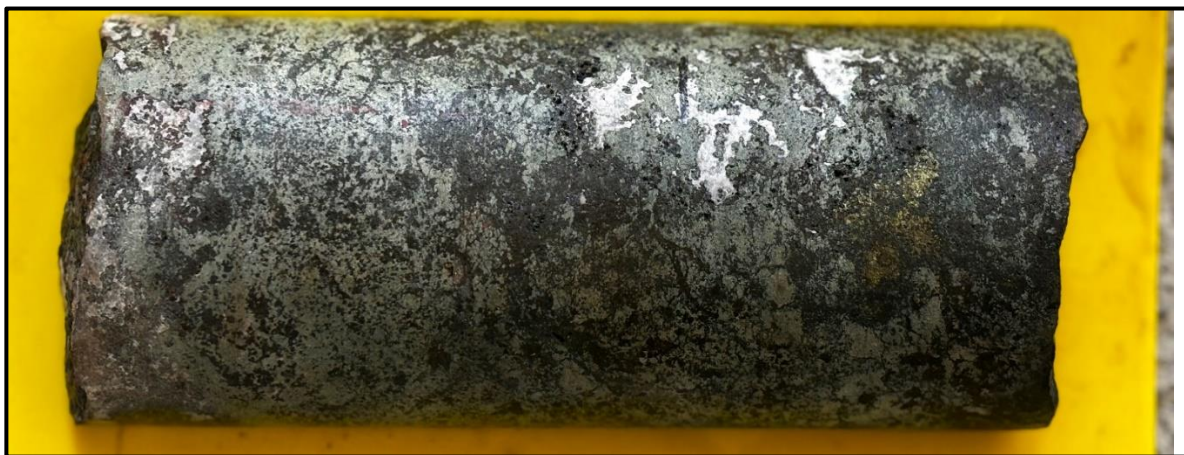
Figure 10. Drill core from 393.5m in ZRSD24148, assaying 4.0g/t Au Eq (0.3g/t Au, 0.2% Cu, 6.2% Zn and 6.1g/t Ag)
