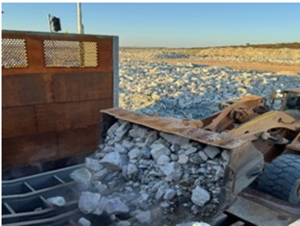
Figure 10: Ore loading into Primary crusher
