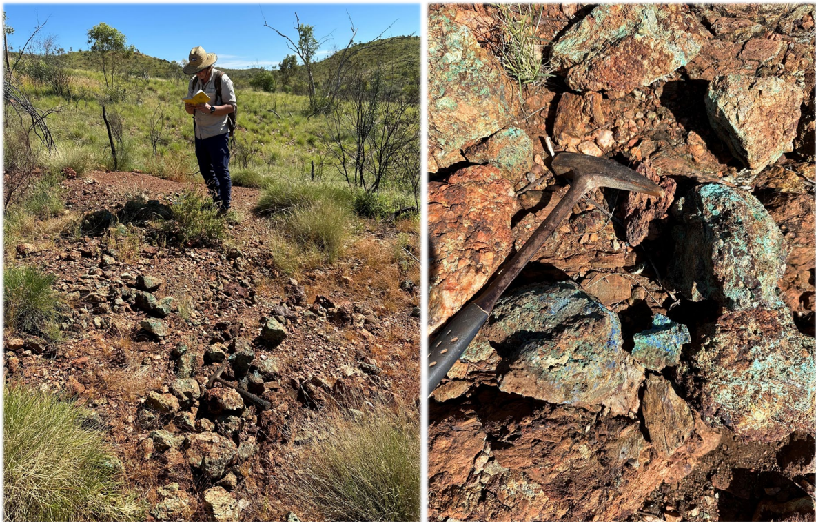
Figure 3. Mohawk Prospect outcropping copper mineralisation (green = malachite).
