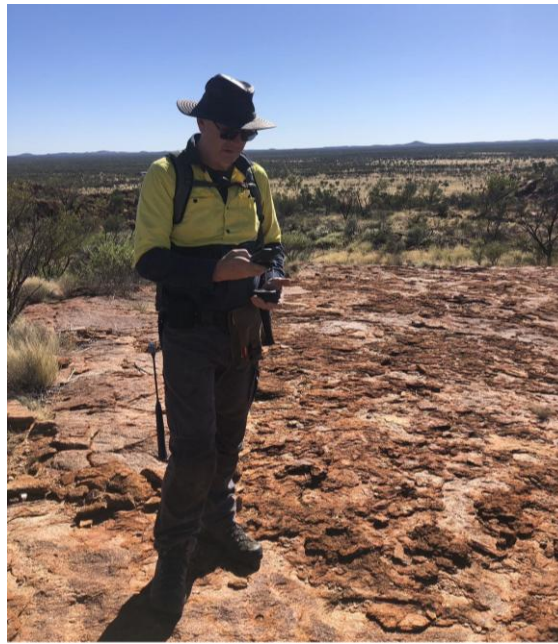
Figure 5: Graeme Fraser conducting field work within Oceana's EL32836, standing with a radioactive reading machine (Gamma-ray ( \gamma -ray) spectroscopy) at the granite tested by Callabona Uranium Limited with shallow diamond drilling
