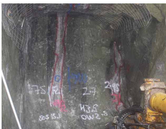
Figure 9 - 1085 Main Lode North - Cut 21 (Split fired cut)
