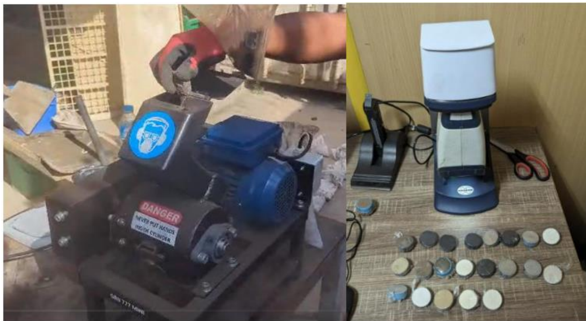
Figure 2: Crusher / Pulveriser and pXRF analysis system set up at Estrella's office in the capital city of Dili
