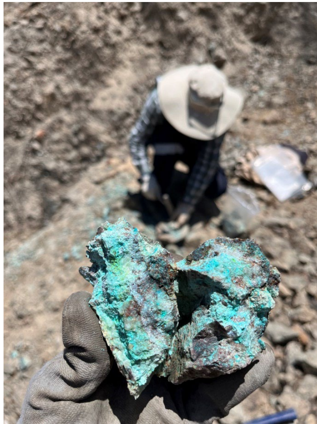
Figure 5: Grab sample 17181 (1.0% Cu) with copper oxides from outcropping historical workings at Cinto Project 4 .
