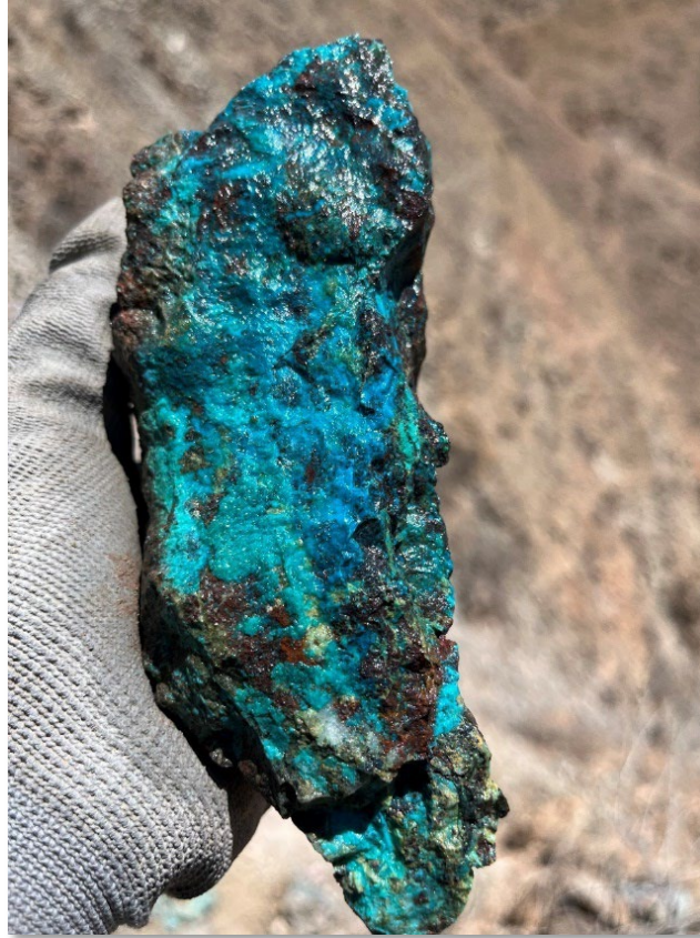
Figure 4: Cinto Project surface grab sample 17142 with visible copper oxides and silicification returned 7.14% Cu 4
