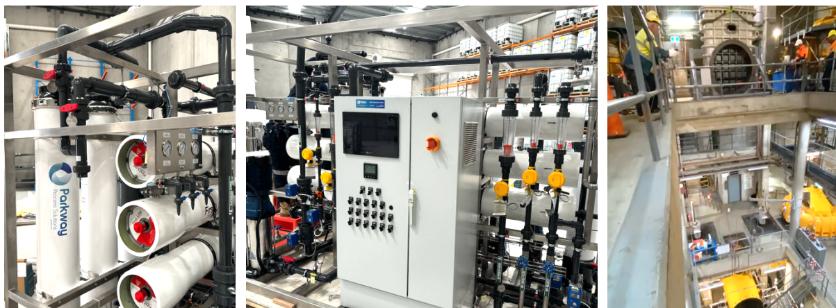
2a: Integrated UF-RO system.
