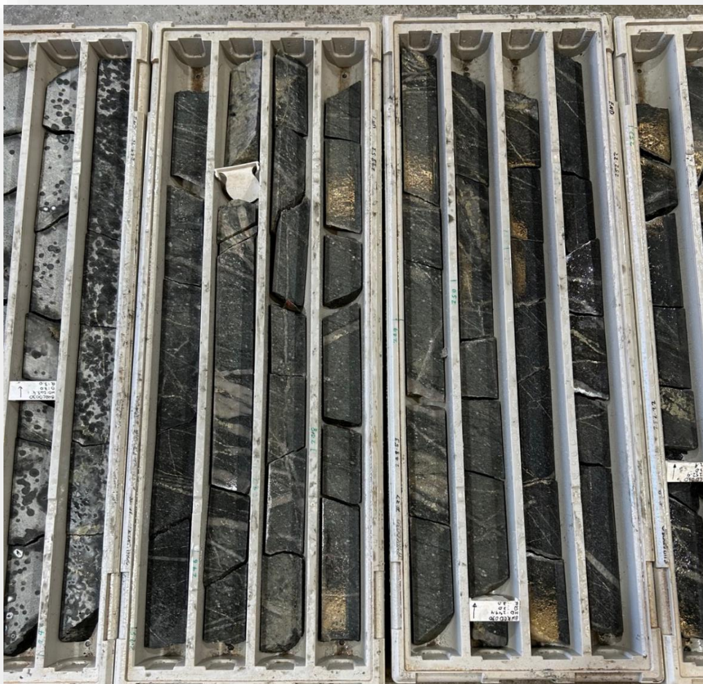
Figure 2: Photograph of core from BHRC030, 123m showing quartz-pyrite veins \pm chalcopyrite-molybdenum
