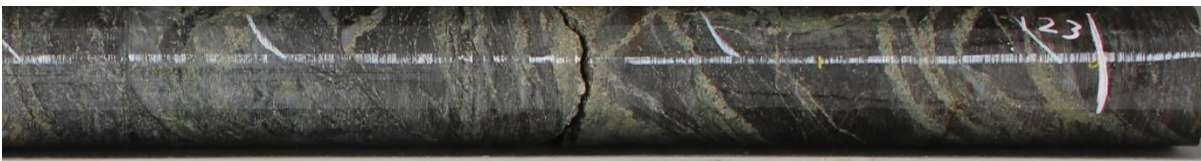
Figure 2: Photograph of core from BHRC030, 123m showing quartz-pyrite veins \pm chalcopyrite-molybdenum
