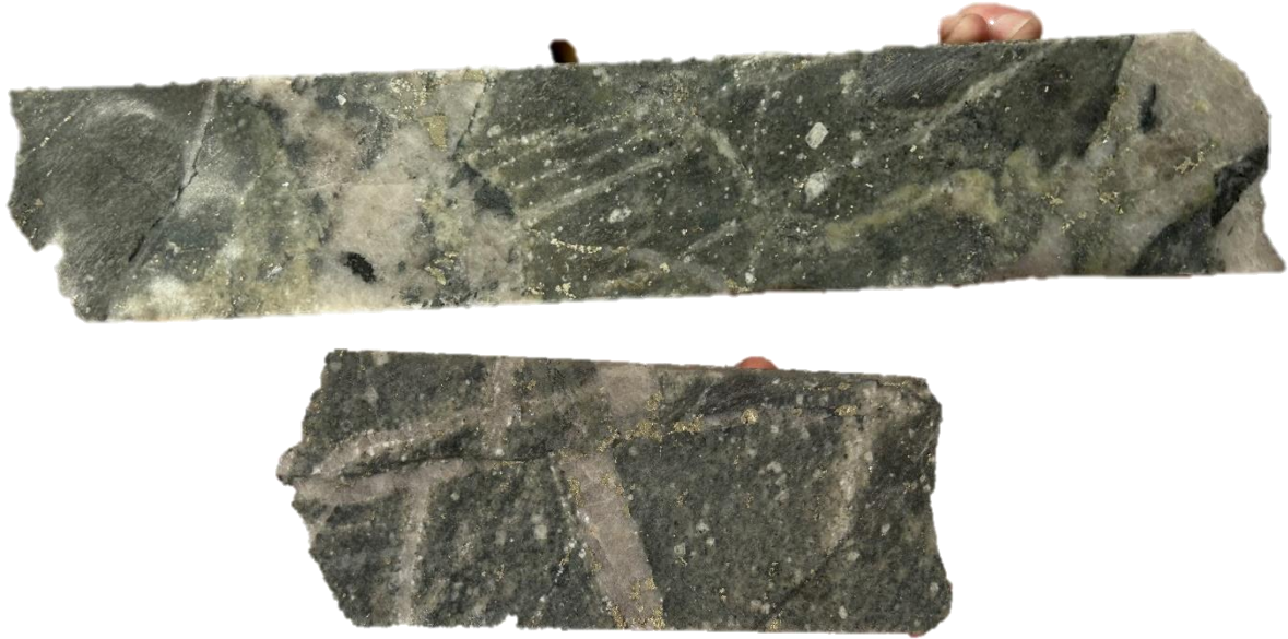
Figure 4: Photographs of core from BHRCD018 showing sulphide minerals hosted in cross-cutting veins
