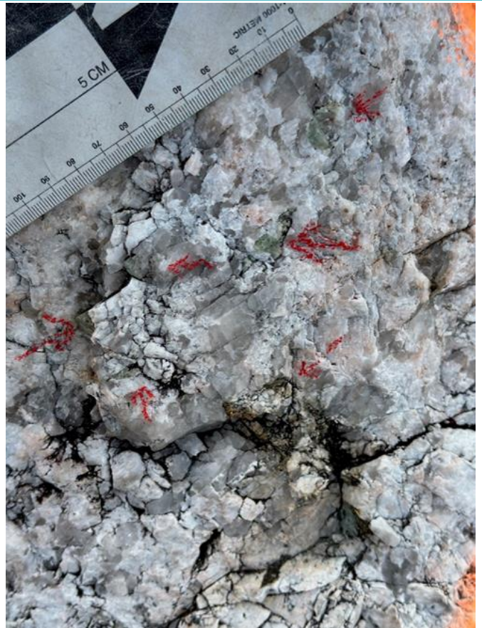
Figure 8 – Raw outcrop with the green mineral returning elevated LIBs readings.
