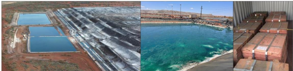
Figure 4 – Stockpiled Material, ILS Pond, and Prior Cathodes Produced at Nifty
