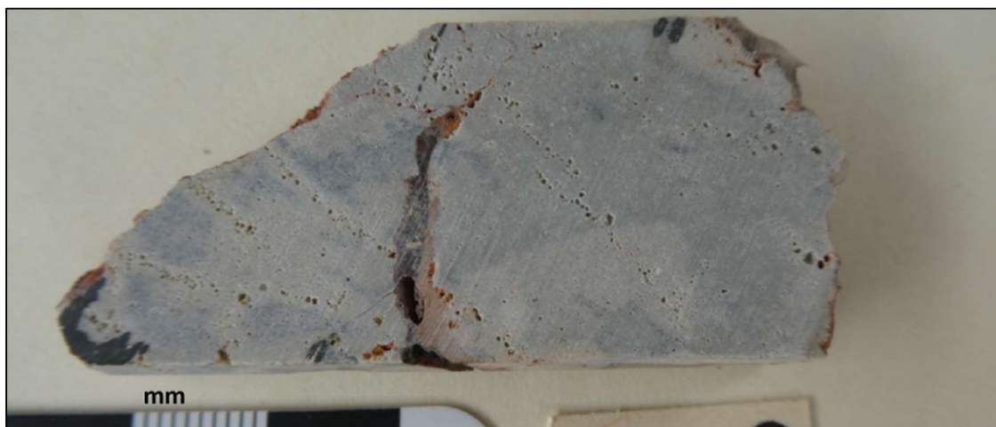
Photo 2 – Slab from Atlantis outcrop of sample KB03118 which returned 0.84g/t Gold 6 , dominated by secondary silica (hydrothermal alteration), containing abundant ex-sulphide coarse voids (up to 1mm) which are flanked by fibrous pressure fringe quartz.
