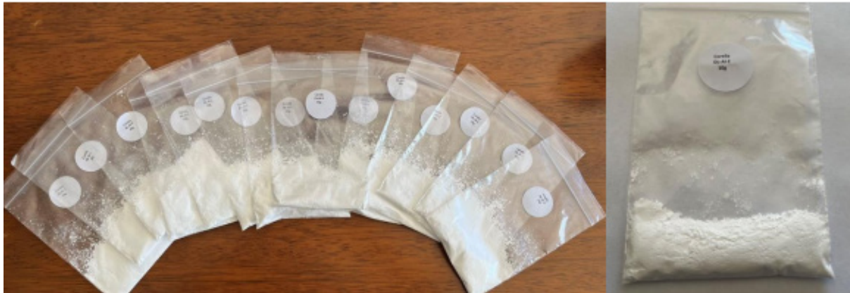
Figure 1: 5N HPA produced using optimised flowsheet from Tampu Kaolin
