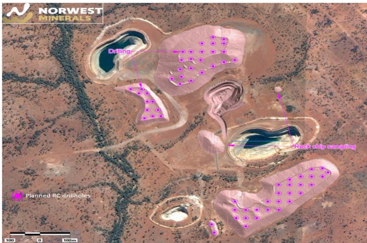
Figure 16 – Newly surveyed waste dumps and open pits mined in 1996-98 and 2002-04 for oxide mill feed. Location of planned RC drill collars to determine the gold content of the dumps are also displayed.
