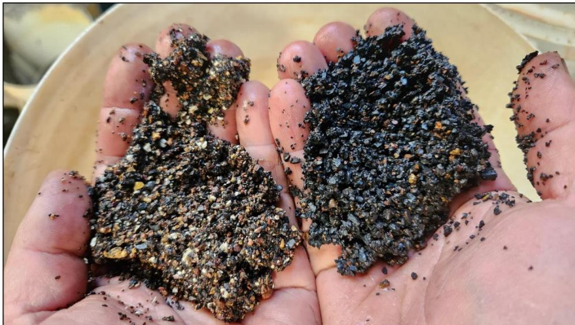
Figure 4: DMS separated material from KR1 showing beneficiated manganese ore on the right side and waste to the left.
