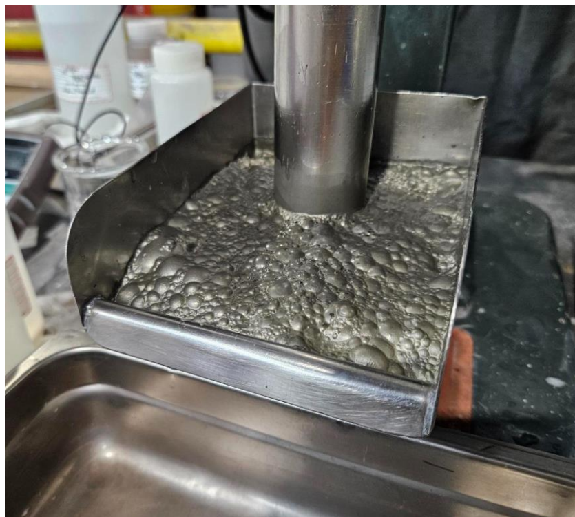
Figure 8: 3rd cleaner sulphide concentrate assaying 29.1% nickel
