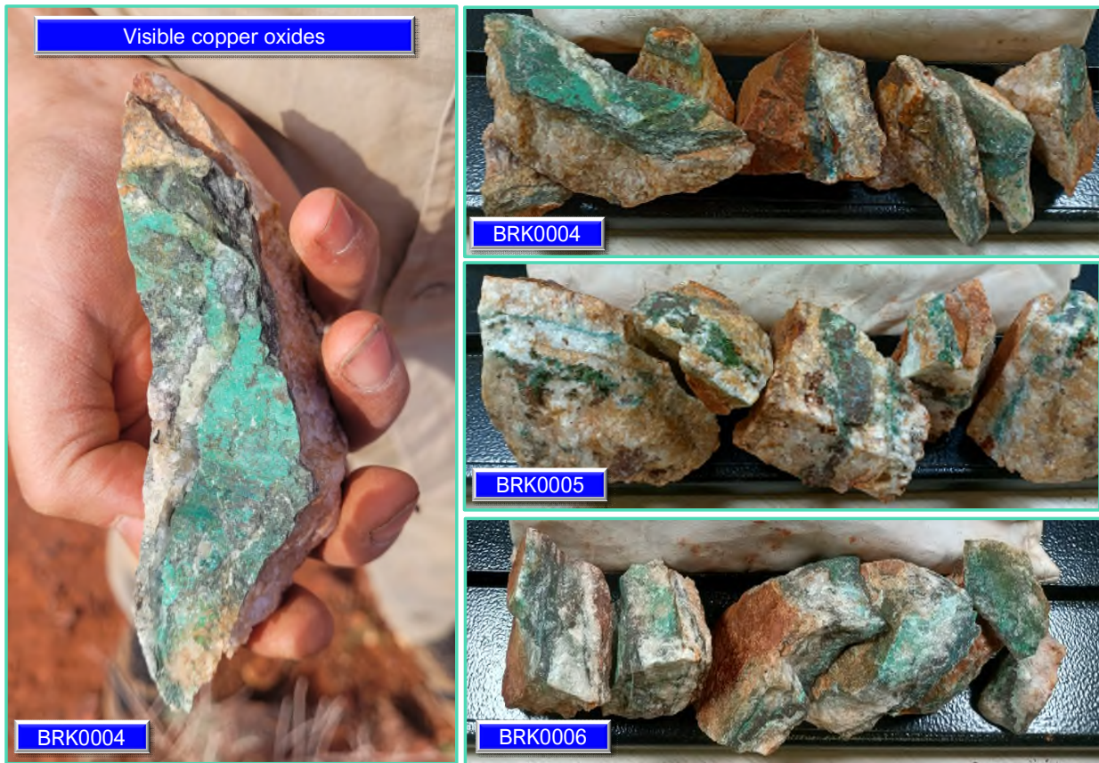
Figure 4. Rockchip photos from Eldinero (E51/1909) showing visible Cu oxide & sulphide mineralisation.
