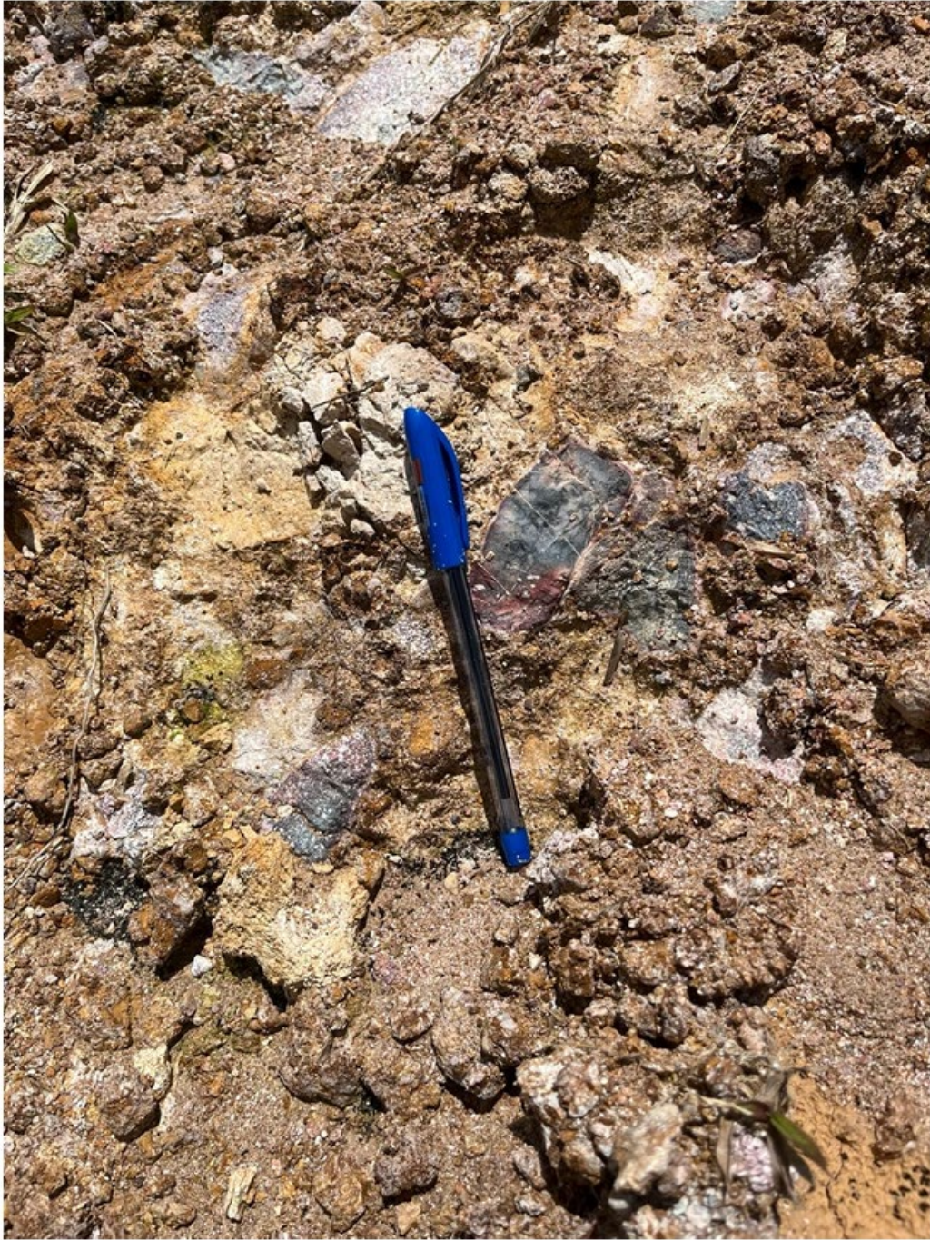
Figure 5 - Recent photo taken by Alice Queen of diatreme breccia is polymict with angular clasts and is matrix supported, with mineralised veining noted cutting across clasts
