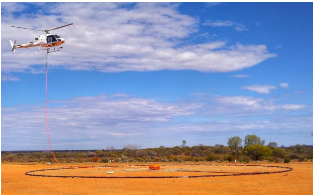
Photos 1: Expert Geophysics TargetEM26 (TIME-DOMAIN EM) SYSTEM and AIRBORNE MAGNETOMETER SYSTEM.
